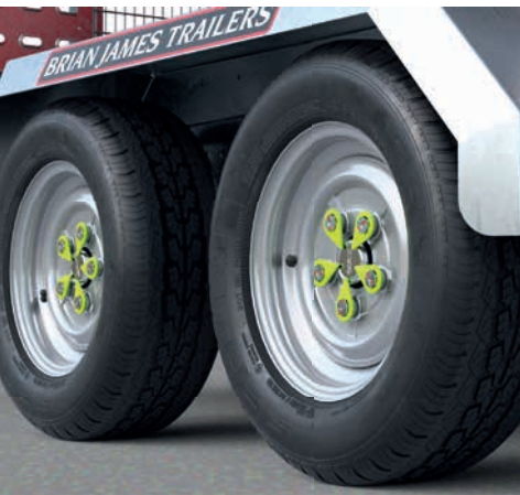
○ Wheel safety indicators Visually reveal whether wheel nut torque has changed once originally set.
