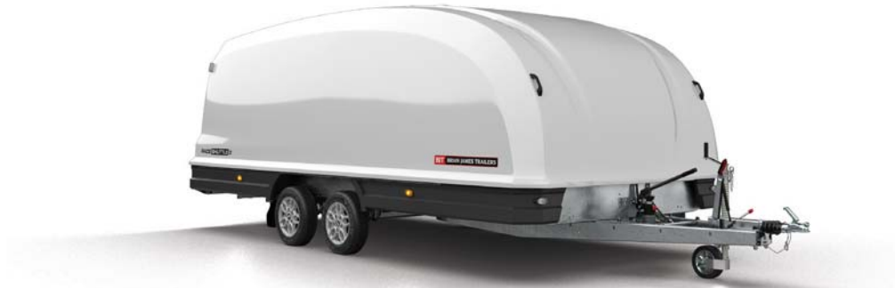
Aerodynamic single piece, clam shell design reduces wind drag and improves towing fuel consumption.
