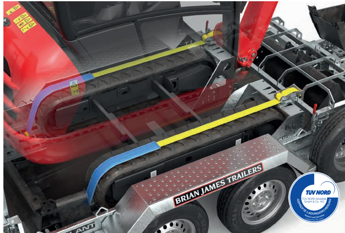
○ TracStrap system The Tracstrap system is unique to Brian James Trailers and the Digger Plant. This in-house designed and manufactured system offers extremely high levels of towing security with minimal effort (TÜV Nord test report 8114838799). The front chocks are adjustable and provide a fixed loading point. Each track is held in place by a 5 tonne rated 50mm wide straps featuring heavy duty wear protectors.
